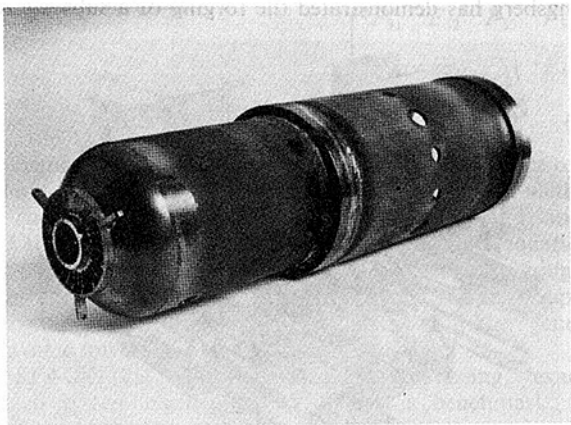
Fig. 5 Rich front end burner developed in atmospheric and full pressure rigs at Kongsberg
